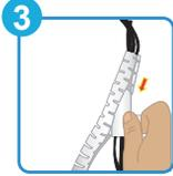
3. Hold the organizer tube and move the device across it. By making this operation, you can put the cables into the organizer tube without any problem.
